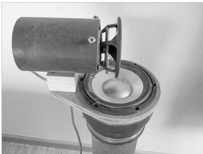
Figure 19: Acoustically coincident layout of woofer and full-range drivers and with cylindrical scattering body behind the full-range.
