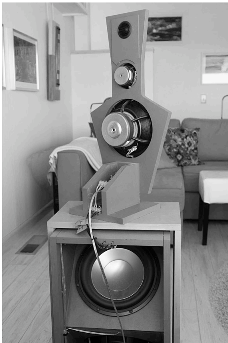
Figure 13: Rear side of open-baffle loudspeaker. Sound radiated to the rear is of opposite polarity to sound radiated from the front. The baffle contour and depth defines the path length and thus the amount of phase shift and the degree to which the rear radiation will cancel the sound in the frontal hemisphere.
